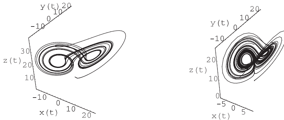
Figure 2: a) Orbit of the Lü system for a = 36, b = 3, c = 19 and the initial condition (-1, 0.1, 4) (left); b) Orbit of the T system for (a, b, c) = (2.1, 0.6, 30) and the initial condition (0.1, -0.3, 0.2) (right).
